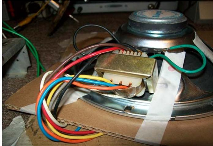
First I need to know the output impedance of a 6V6 tube. After doing a little research (RCA Tube Manual) I determined that the 6V6 when used as a Single Ended output tube was about 5,000 ohms impedance. Now all I need to know is which wires to use on the input of the audio transformer to match the 5,000 ohms to the 8 ohms on the speaker side of the transformer.
